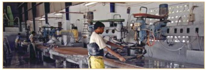
Machines: 4 Circular Saws, Processing up to 100 cm i.e. 65 - 100 x 180 - 340 cm. 1 Circular Saws, Processing up to 100 cm i.e. 100 - 125 x 240 - 340 cm.
